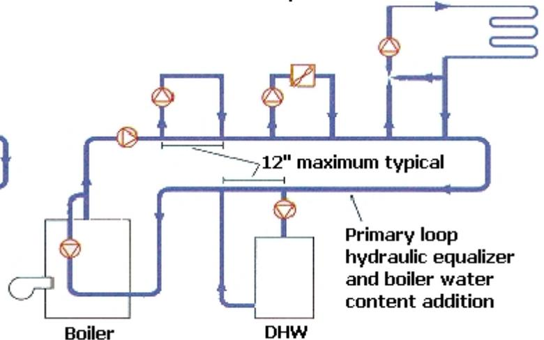
The primary/secondary pumping approach is low cost; piping is schematically simple, demanding low labor. There are no circuit backflow problems, check valves or pressure differential valves.
