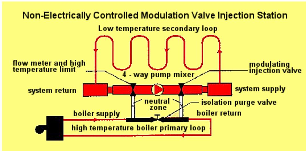
this station is ideal, dramatically reducing distribution piping cost and eliminating a multitude of circulators and electronic controls.
