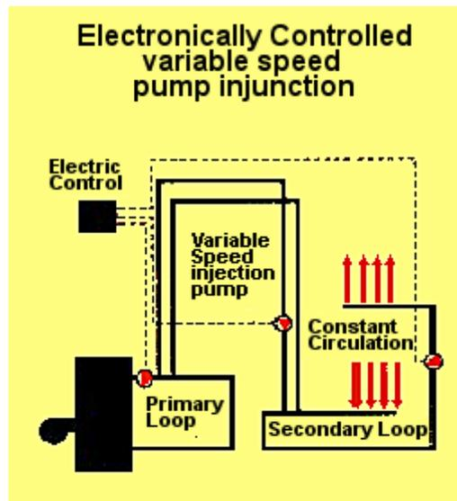
valve position. In the case of electronic injection, the injection point can be anywhere on the secondary loop within the suction side of the system circulator. Here the injection volume is controlled by a variable speed injection circulator.
