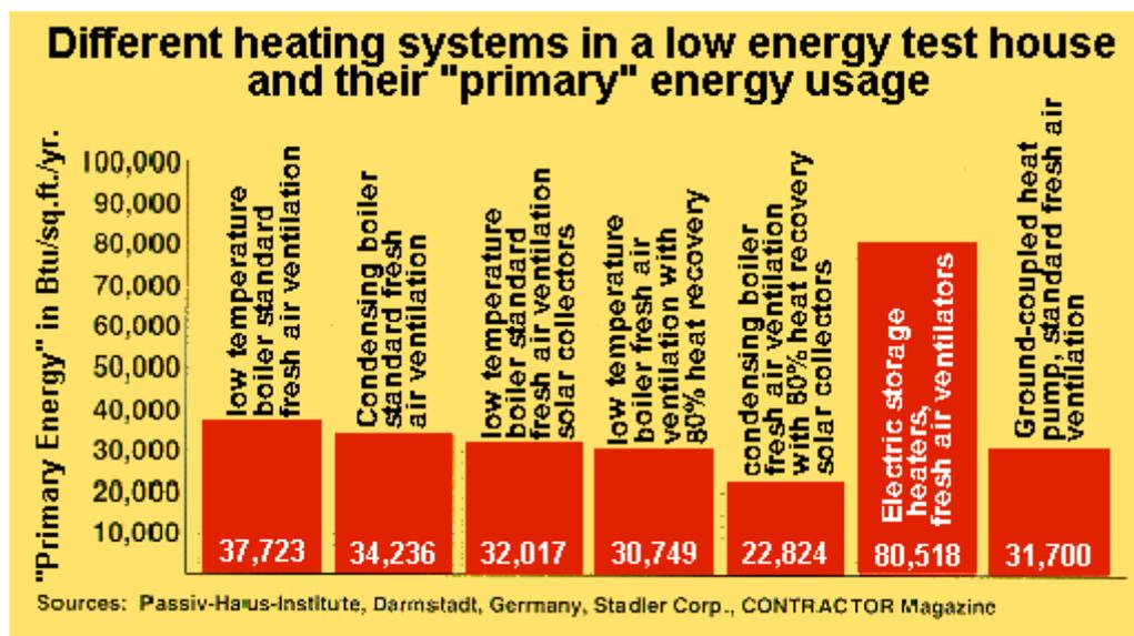
A research institute in Germany tested a variety of heating systems' energy usage to see which system would be the most efficient. The winner was a condensing boiler with a heat recovery ventilator and solar domestic hot water.
